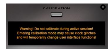
To calibrate an Atomic Master Clock, ensure atomic signal is fed to the OCX HD's Atomic Input, the Atomic Clock is warmed up and the OCX HD Atomic Clock Indicator is lit.
