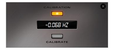
3. Repeat the procedure as many times as necessary so that the number becomes as close as possible to 0 and relatively stable (it may have small deviations of a few seconds). To exit Calibration Mode, press the **X** button.
